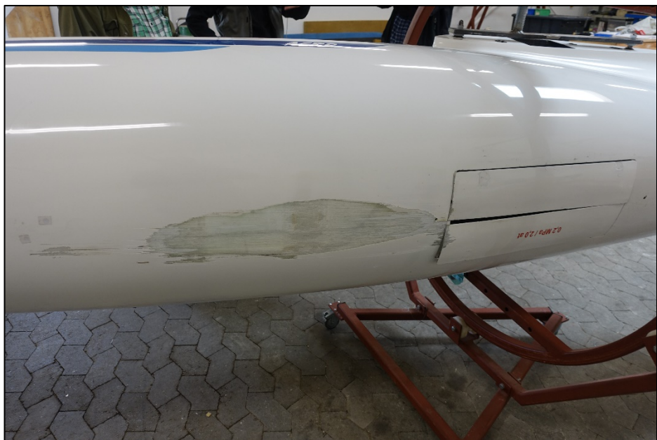
Photo no. 2: Abrasion damage to the lower part of the fuselage skin, frames and wheel doors.
