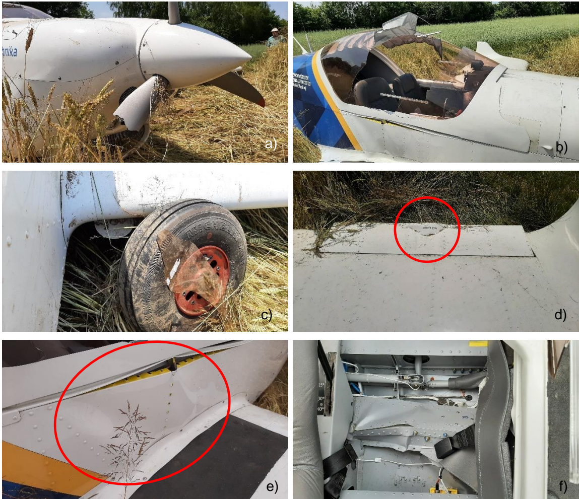
Fig. 1. Damage to the aircraft: a) propeller, b) broken windshield, c) damaged main gear, d) deformed left aileron, e) corrugated structure of the starboard, f) torn fuselage reinforcements for main landing gear [source: SCAAI]
