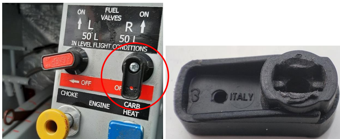
Fig. 2. Damaged knob of the right tank valve. On the right – the enlarged view of the knob (view from the bottom), grooves for the spindle are well visible [source: SCAA]
