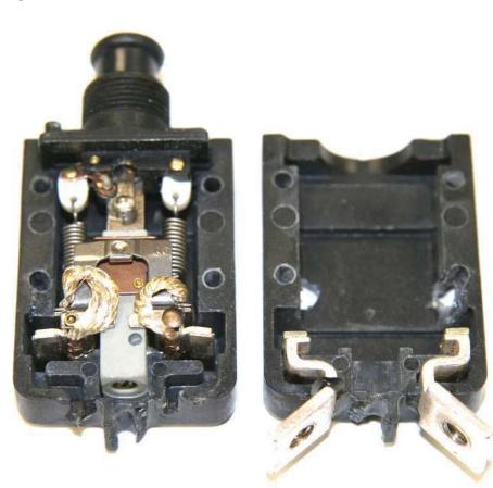
Figure 15: BACC18X25 housing open.
