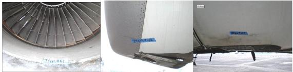
Figure 4. Damage to the right engine nacelle – from the left: fan inlet inside, bottom part, thrust reverser. (Source: Boeing)
