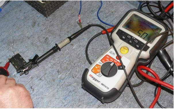
Fig. 12. Measurement of insulation resistance of C829 circuit breaker
