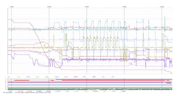
Figure 14. SP-LPC approach to landing – as recorded by the SSFDR.
