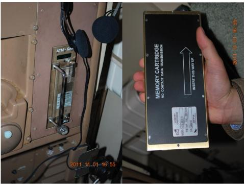
Figure 9. QAR recorder from SP-LPC and its memory cassette. (Source: SCAAI)
