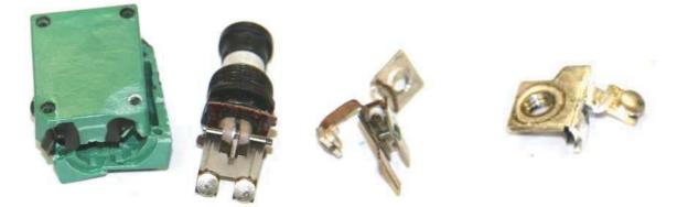
Figure 22: The BACC18Z7R circuit breaker disassembled.
