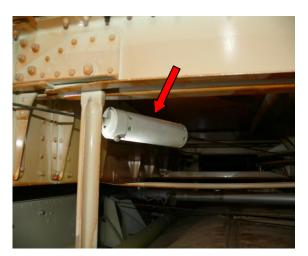
Figure 21. Load limiter of the alternate landing gear extension system (right main gear). (Source – SCAAI)
