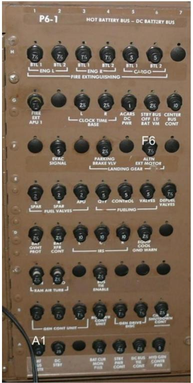
Fig. 1. P6-1 panel. C829 BAT BUS DISTR on A1 position
