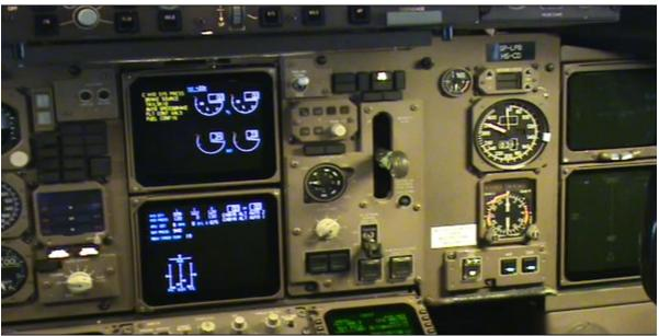
Fig. 2. Test of landing gear extension, C829 (A1) in OFF setting
