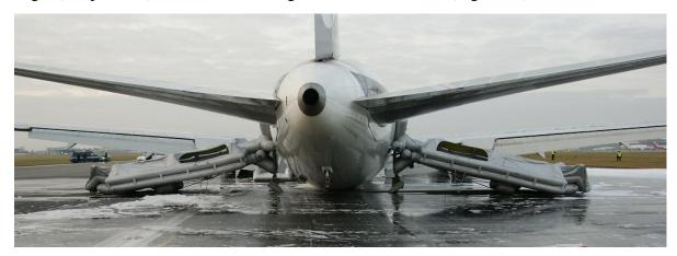
Figure 16. Setting of the rear slides of SP-LPC airplane after emergency landing.
