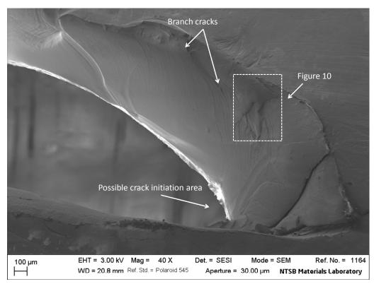
Figure 9. SEM image of center section of secondary fracture surface and crack initiation area.
