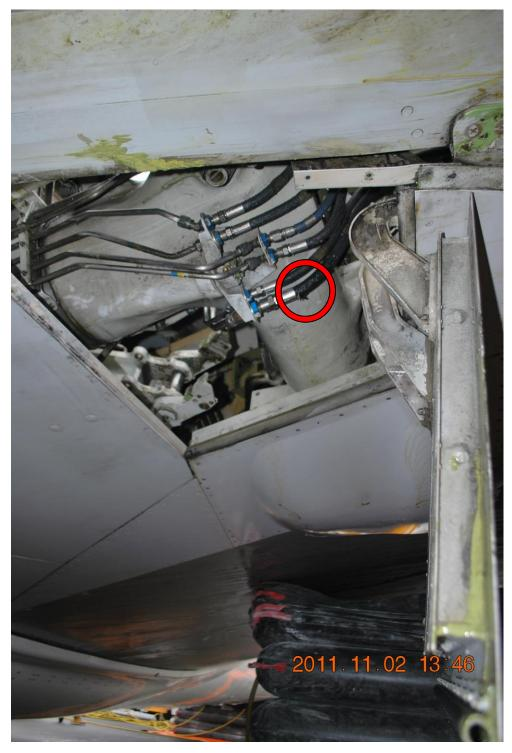
Figure 22. Damaged hydraulic hose (marked with red circle) on SP-LPC right main gear. (Source – SCAAI)
