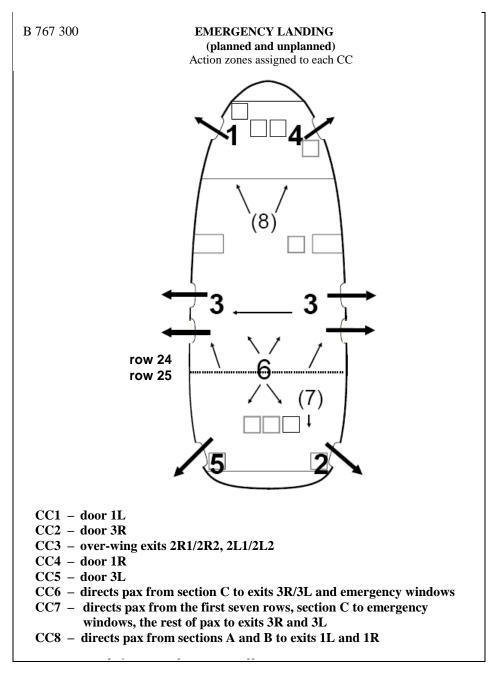
Figure 17. Action zones of the cabin crew during emergency landing.
