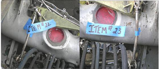
Figure 2. Damaged struts of the main landing gear hatch door (left and right). (Source: Boeing)
