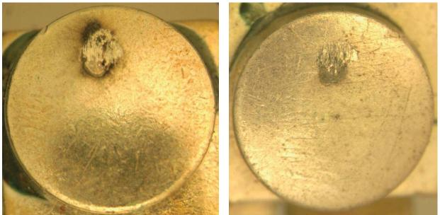
Figure 23: BACC18Z7R fixed contact 1.
