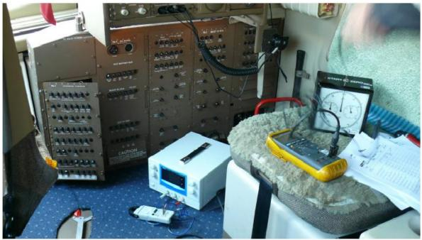
Fig. 17. Test set for measurement of the trip time of the circuit breakers
