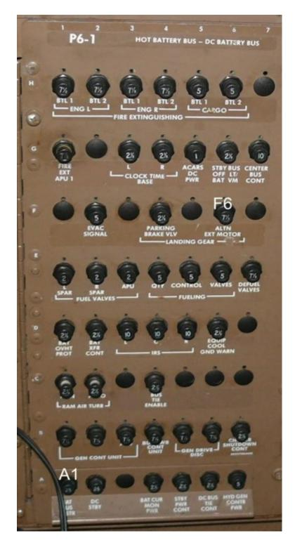
Figure 6. P6-1 panel. A1 - C829 BAT BUS DISTR circuit breaker and F6 – C4248 LANDING GEAR – ALTN EXT MOTOR
