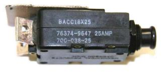
**Figure 8:** BACC18X25 circuit breaker in the "as received" condition.
