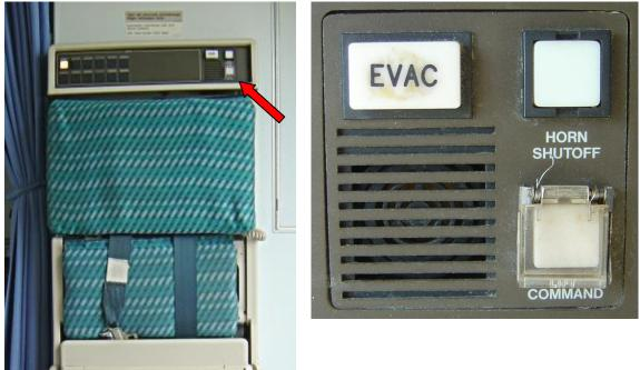
Figure 6. Evacuation signaling system over CC5 seat.
