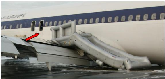
Figure 5. Evacuation slide on the let wing and locked drop step.
