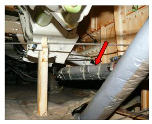
Figure 19. Load limiter of the alternate landing gear extension system (nose gear). (Source – SCAAI)
