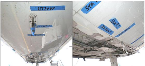
Figure 1. Damage to the lower part of the fuselage in the area of section 46 – front view and close up. (Source: Boeing)
