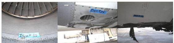
Figure 3. Damage to the left engine nacelle – from the left: fan inlet inside, bottom part, thrust reverser. (Source: Boeing)
