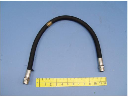
Figure 1. Overall photograph of accident hydraulic hose.
