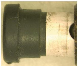
Figure 28: BACC18Z7R button and shaft.
