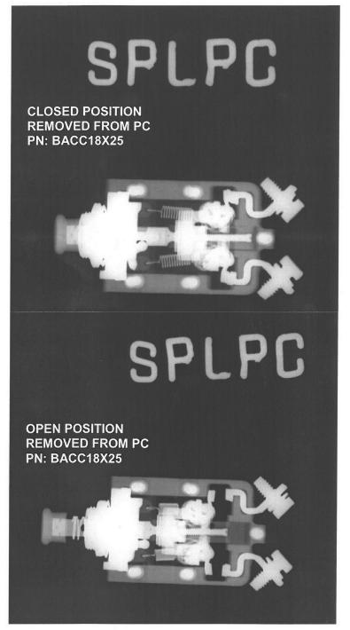
Fig. 8. X-ray picture of C829 circuit breaker
