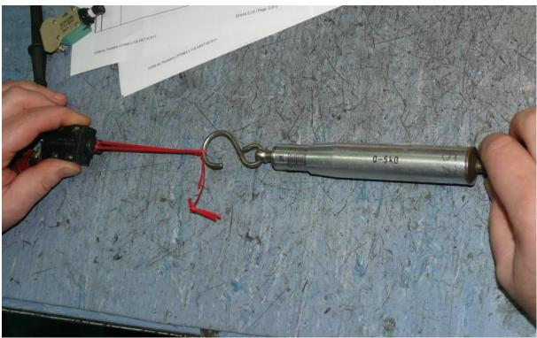
Fig. 11. Measurement of pull-out force (OFF setting force) of C829 circuit breaker
