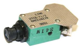
**Figure 7:** BACC18Z7R circuit breaker in the "as received" condition.
