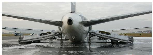
Figure 4. Position of the aft slides of SP-LPC airplane after gear up landing.
