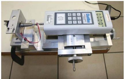
Figure 12: Operating force test setup.
