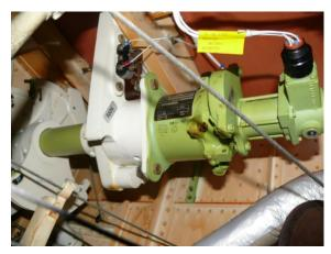
Figure 18. Electric actuator of the alternate landing gear extension system (Source - SCAAI).
