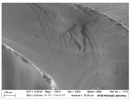
Figure 10. Close-up SEM image of branch cracking and directional crack markings.
