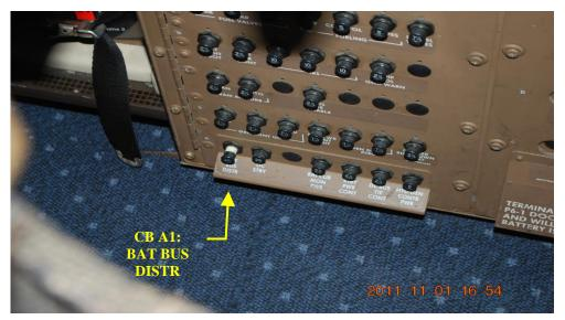
Figure 25. P6-1 panel in the cockpit (section with C829 circuit breaker). (Source – SCAAI)
