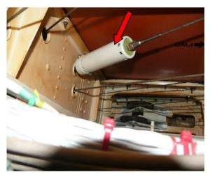
Figure 20. Load limiter of the alternate landing gear extension system (left main gear). (Source – SCAAI)
