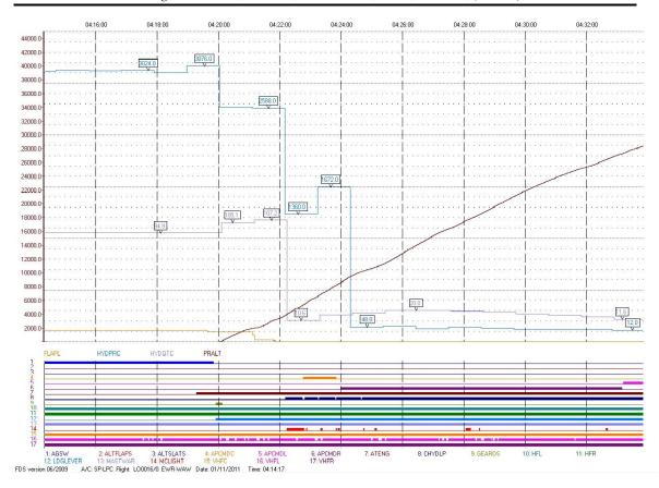
Figure 13. Pressure drop in the center hydraulic system of SP-LPC after its take-off - as recorded by the SSFDR.
