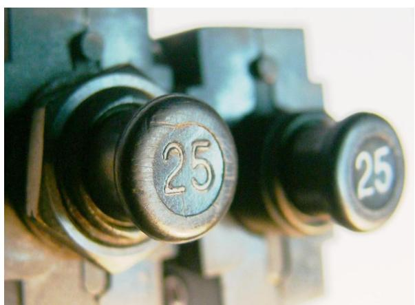
Fig. 9. Buttons of C829 circuit breakers (left – from SP-LPC, right – a new one)
