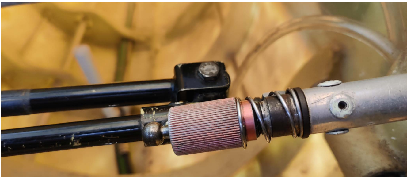
▲ The loose L'Hotellier control connection. (Source: pilot)
