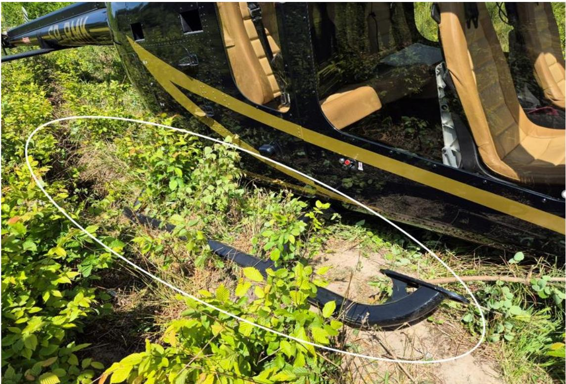
Figure 4. Damage to the right landing skid of the helicopter.
