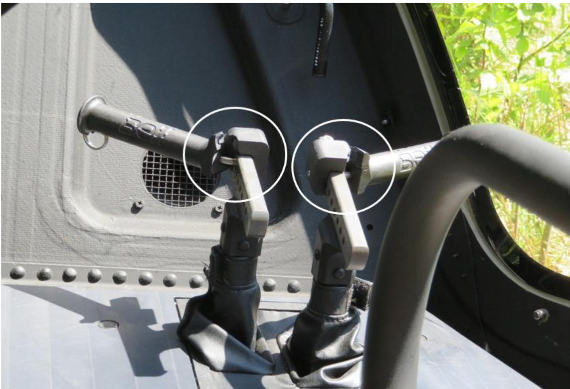
Figure 6. Damaged pedals on the side of the pilot flying.
