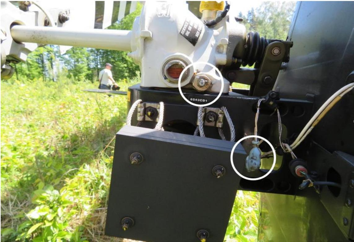
Figure 5. Damaged oil sight glass, torn off control cable chip detector in the angled gearbox.
