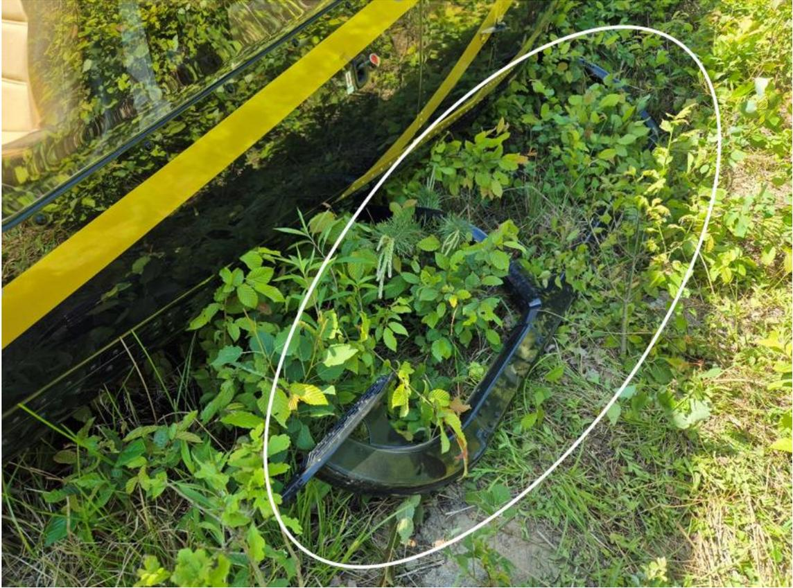
Figure 3. Damage to the left landing skid of the helicopter.
