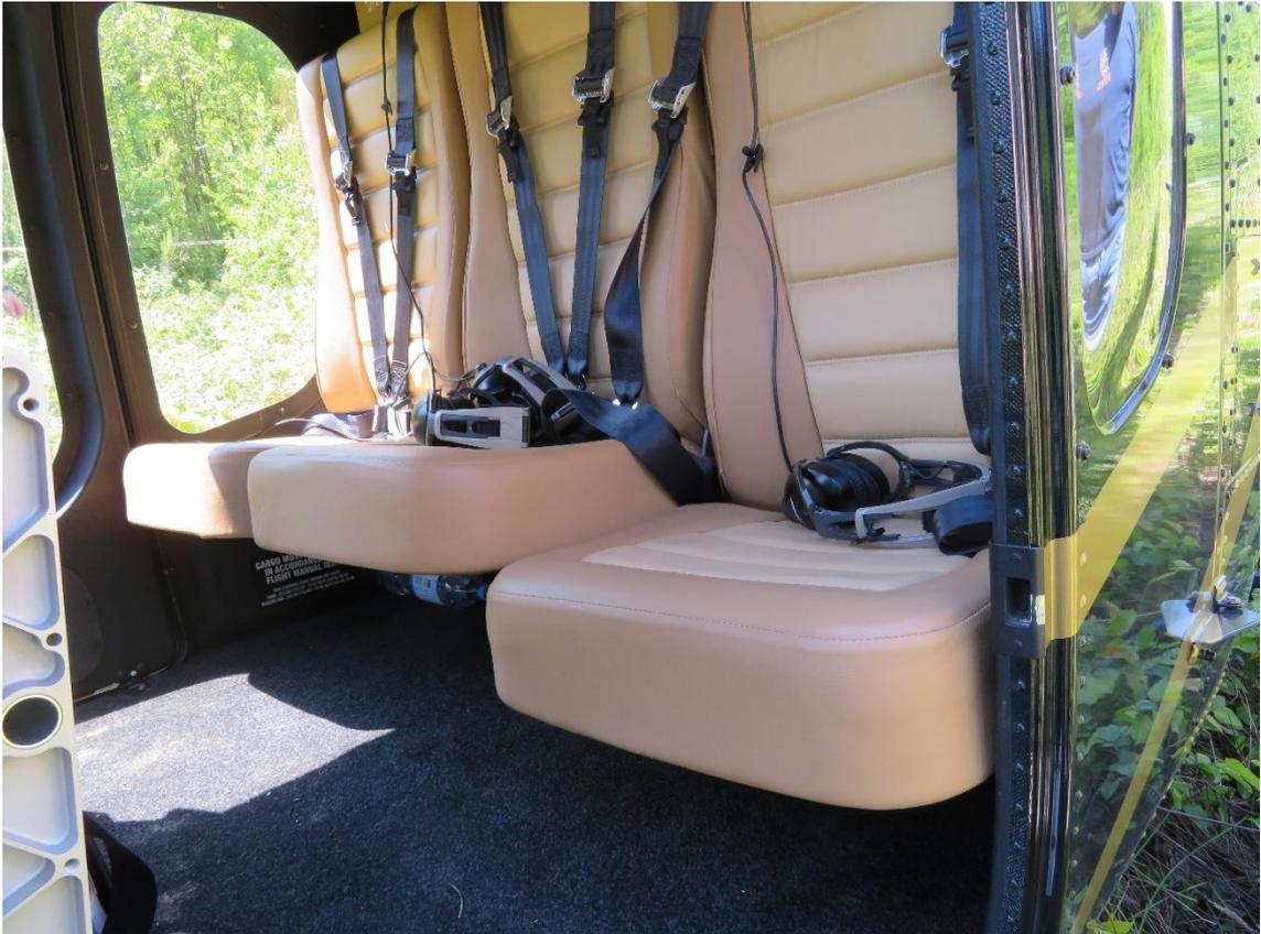
Figure 7. Rear passenger seat after operation of the energy absorption system
